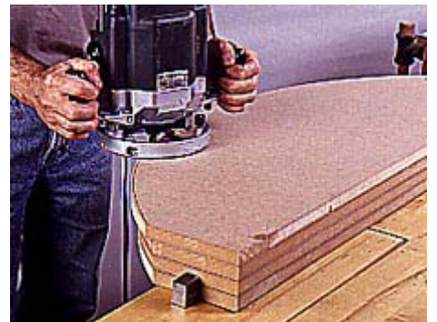
2 The remaining pieces of the form are trimmed to size using the template, router and flush-trimming bit.
