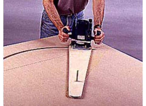
1 Make the bending form template with a plunge router on a trammel arm. Cut an arc in a sheet of MDF.
