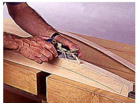
13 Cut the outside curve on the leg. Clamp it to the bench, and smooth the curve with a block plane.
