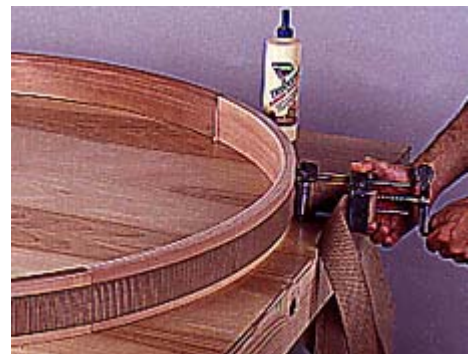
8 Glue and clamp the apron sections together using a strap clamp. Check its diameter at several points.
