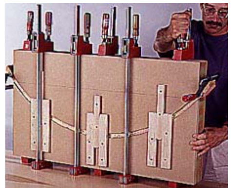
5 Clamp the laminate strips at either end to keep them from shifting. Apply pressure with equally spaced clamps.
