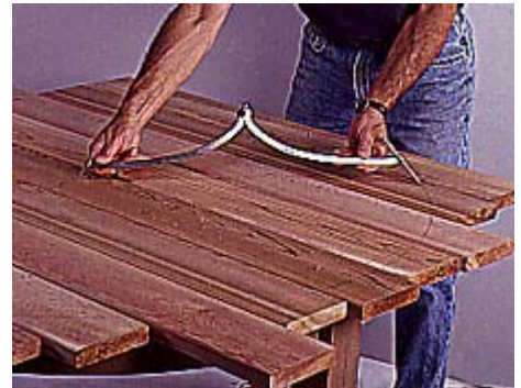
11 Space the boards equally, and screw them to the crossrail. Draw the outline of the top on the boards.
