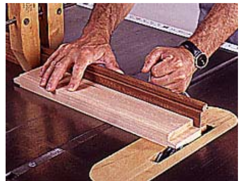
16 Clamp a stop to the miter gauge fence. Use a dado blade to cut the tenons on the rails, stretchers and back slats.
