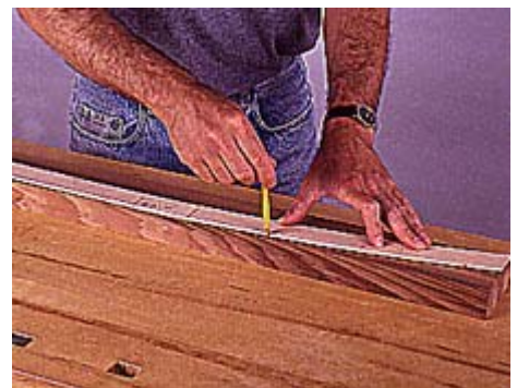
12 The first step in building each chair is to make a template for the rear leg, and trace it on the leg blanks.
