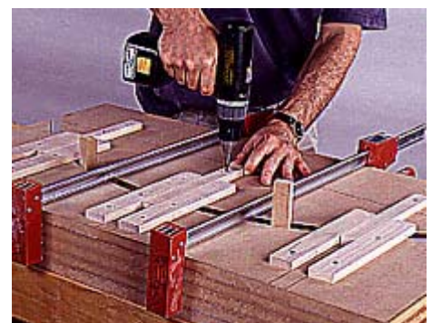
3 Use 3/4-in.-thick spacers between the bending form pieces. Clamp the form pieces together and fasten alignment strips.
