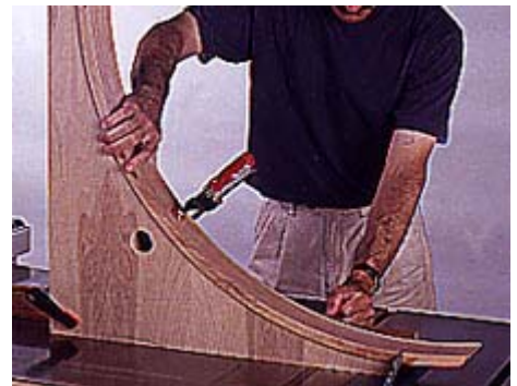
6 Make a cradle. Then crosscut the apron blank to finished length. The apron length and cradle arc length are equal.
