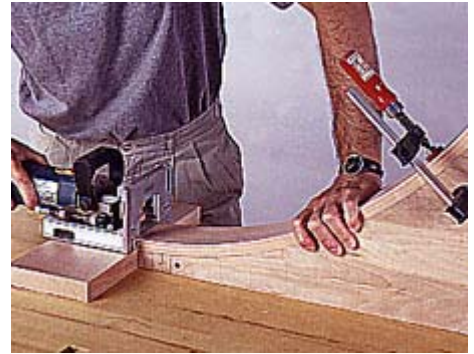
7 Transfer the cradle to a bench, and use it to hold the apron section in place while cutting the biscuit slots.
