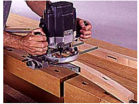
14 Use a plunge router with its fence positioned on the leg's straight face. Cut the side rail and stretcher mortises.
