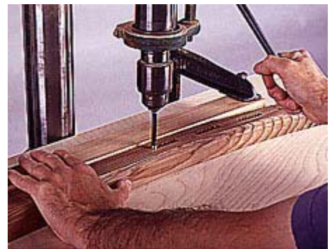
15 Remove the bulk of the side rail mortises on the drill press. Chisel the mortise sides and ends square.
